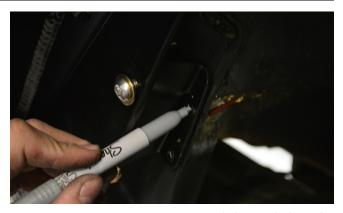
14. Use a fine-tip felt marker to mark the two holes to be drilled in the upper-rear corner, where the two remaining (non-countersunk) holes are, in order to install the Rear Inner Fender Bracket.
