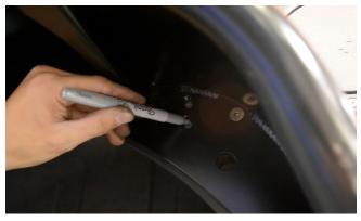
**15. Remove the Crusher Flare and** drill the four holes marked in Steps 8 & 9, to 5/16". On the two holes for the Rear Inner Bracket, drill through both the outer and inner layer of sheetmetal (about an inch apart). Make sure the drill is held perfectly perpendicular to the sheetmetal to ensure proper alignment of the holes through the inner sheetmetal. Use touch-up paint to protect the cut edges of the drilled holes from future rust.
