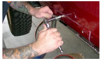
8. Once the nut-sert has seated correctly, loosen the bolt then remove it and the rest of the tool from the nut-sert. Install a new nut-sert onto the tool, oriented the same as the last, and set it aside until your next nut-sert installation.
