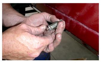
**9. With the tool removed, inspect** the nut-sert to make sure it is properly seated and that the surrounding sheet metal isn't excessively deformed. Note that some deformation of the sheet metal is normal, and that it will be covered by the part after installation.
