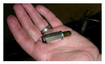
7. Use an open end wrench to hold the coupler nut stationary while turning the head of the bolt clockwise with a ratchet (or small impact wrench) and socket. As you turn the ratchet, the bolt will draw the far end of the nut-sert toward the inside of the sheet metal, gripping it with the knurled outside edge of the nut-sert as it deforms. Continue to turn the ratchet until the nut-sert is fully seated. DO NOT OVER-TIGHTEN as you can damage the nut-sert, or cause it to lose its grip.
