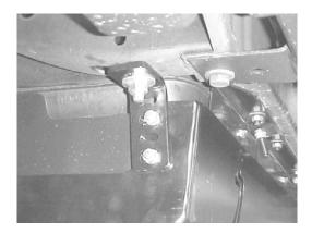
**Step 9:** You may find that you need additional exhaust system clearance as shown in the photo below left. Simply bend the exhaust hanger bracket shown below right to gain this clearance. You can also remove the threads that are protruding past the nut with a hacksaw.
