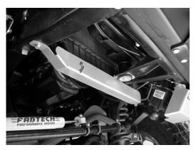
**Step 3:** Align the radiator guard with the lower tank of the radiator. Mark and then drill a 5/16" hole into the passenger side of the frame using the hole in the guard as a guide. **Note:** The tab on the guard will not sit flat on the chassis until after the bolt is tightened. **Note:** You may find it easier if you first mark the hole location and then remove the guard to drill the hole.
