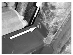
**Step 4:** Drill a 5/16" hole into the frame cross-
