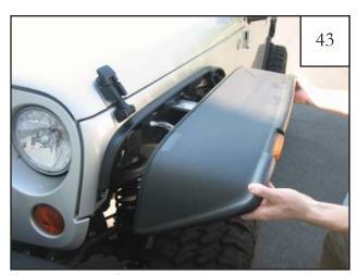
Place the outer flare over the inner pieces and push until snug against the sheet metal. Make sure that the side marker light wires are inside the flare. Make sure splash shield is tucked behind flare.
