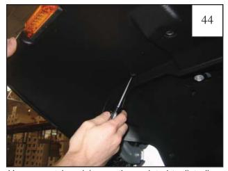
Use a scratch awl (or another pointed tool) to line up the speed clips with the outer flare holes (7 locations). If needed, use a flashlight to better locate the speed clips.
