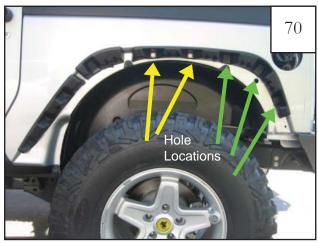
Secure inner piece D6 (and P6 for passenger side installation) to the sheet metal using the following **4 STEPS: Step 1** Position inner piece on fender, aligning with existing factory holes in sheet metal.
