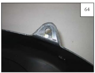
Place a grease pencil mark 1/8" below the hole on the rear mounting tab.
