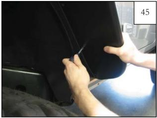
Hold flare in place on fender and start a pan head screw into each hole location and through speed clip on inner structure and metal frame angle support bracket (7 locations). Do not tighten.
