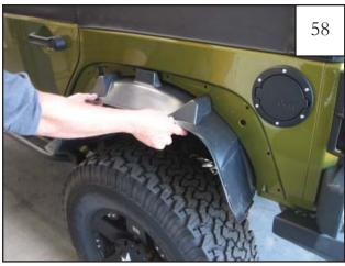
Hold the splash shield in place using supplied 1/4" Panel Retainers through factory holes halfway. Do not fully install Retainers, leave them half out. They are only used to hold splash shield in place for marking. See step 76 for locations.
