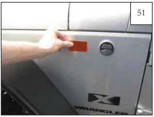
Attach one side reflex reflector to the side of the vehicle by peeling off the adhesive backing and pressing it firmly onto the cleaned vehicle surface. NOTE: Once reflector has adhered it cannot be repositioned.
