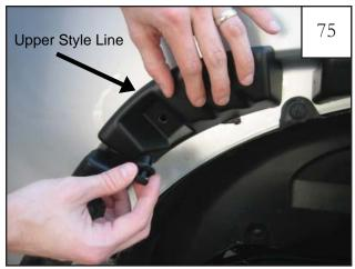
**Step 2** While holding the inner piece in place, install a plastic push retainer. *Inner piece should rest along upper style line of sheet metal radius and not below it:* see step 22.
