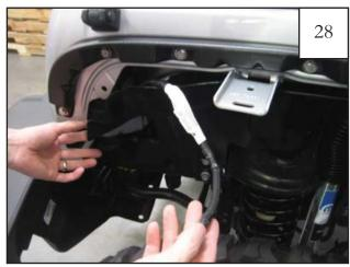
Reinstall light connector removed in step 5. Position inner splash shield for reinstallation, making sure that side marker light wires are outside of splash shield.
