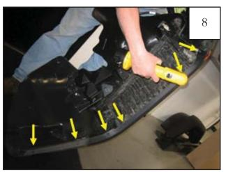
Use a drill with 5/16" bit to drill through six plastic rivets along edge of flare/splash shield. Discard flare. Save splash shield for reinstallation.
