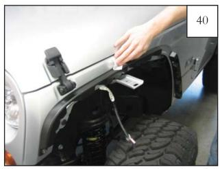
Use one supplied alcohol prep pad to clean the sheet metal above each inner piece in preparation to tape the edge trim to the sheet metal. This must be done for proper flare installation.
