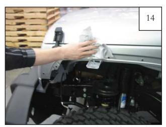
Thoroughly clean the exposed metal fender with a damp cloth and dry.
