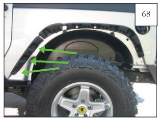
Secure inner piece D5 (and P5 for passenger side installation) to the sheet metal using the following **2 STEPS: Step 1** Position inner piece on fender, aligning with existing factory holes in sheet metal.
