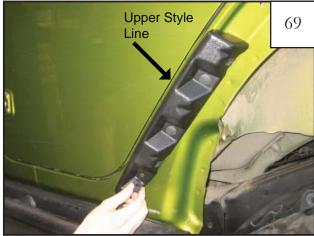
Step 2 While holding the inner piece in place, install a plastic push retainer in each hole location. *Inner piece should rest along upper style line of sheet metal radius and not below it:* see step 22. NOTE: Foam insulation may need to be trimmed out of the holes.
