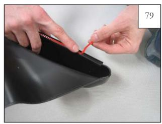
Peel back 1-2" of red liner on each end of the edge trim and bend toward the outside of the flare.
