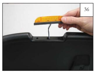
Position the supplied side marker light onto the outer flare piece, threading the wires through the *center* predrilled hole.
