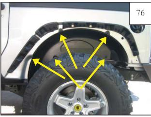
Reinstall modified splash shield using supplied 1/4" Plastic Retainers (5 locations).
