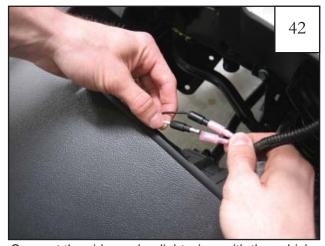
Connect the side marker light wires with the vehicle wires by attaching the male connectors to the female connectors. Test the connection by turning on the front marker/parking lights. Switch connectors if necessary.
