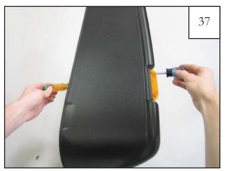
Secure the side marker light to the outer flare with 8-32 screw, 8-32 nut, and washer using a #2 Phillips bit and a 11/32" socket with 8" extension (2 places). NOTE: If you are having trouble putting the washer and nut on the screw, use needle nose pliers.
