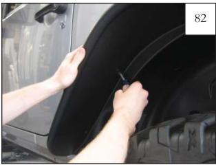
Hold flare in place on fender and start a pan head screw into each hole location and through the speed clip on inner structure (6 locations). *Do not tighten.*
